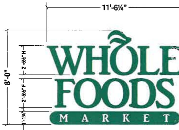
**B** ONE(1) L.E.D. ILLUMINATED CHANNEL LETTER DISPLAY, RACEWAY MOUNTED • FRONT VIEW
