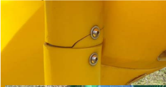
Broken mounting surface on slide
